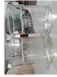
Lime achieved 57% hardness removal at pH 10, while the lime–PACL combination (pH 10.5, 28.5 ppm PACL) reached 66.7% removal with turbidity below 2 NTU. Excess PACL reduced efficiency due to pH drop, and the best results occurred when PACL was added after 20 minutes, showing this method as a low-cost option for surface water softening.
